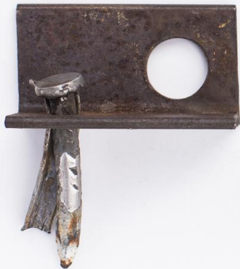
Original Warren Harding bolt from The Nose with home-made hanger
