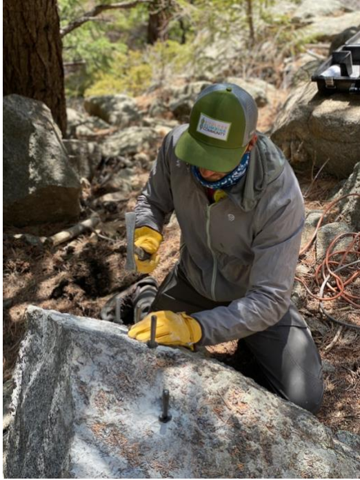
Figure 2- BCC staff using feathers and wedges to quarry stone.
